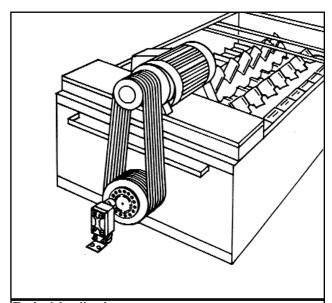
Typical Application: Grinding and blending of dried caked waste material for safe disposal requires 24 hour continuous operation of pug mill. The A1500 or A2500 monitors the driven shaft to indicate broken or slipping drive belts.
